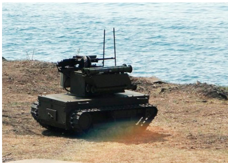
The Platforma-M variant of the Multifunctional Utility/Combat support/Patrol. Serially produced by the Russian Army. Fra en.wikipedia.org - Military robot
